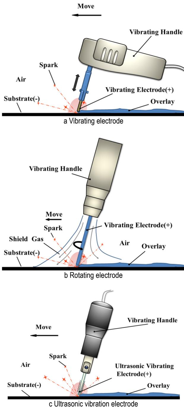
Fig.1 – Process diagram of electro spark deposition
